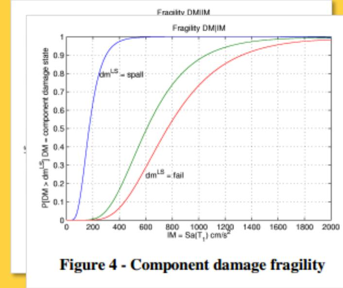
**Figure 4 - Component damage fragility**
