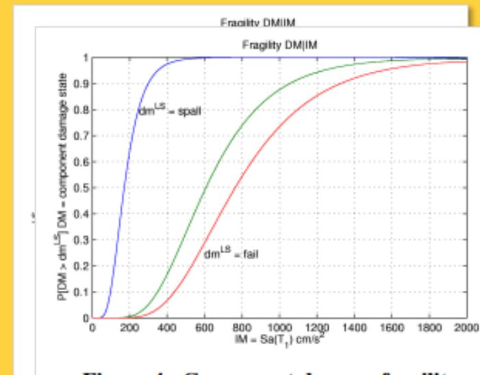
**Figure 4 - Component damage fragility**
