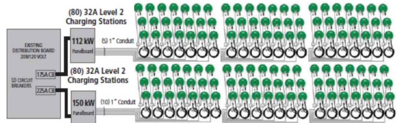
(160) 32A Charging Stations on 262 kW total capacity using UL916 Adaptive Load Management
